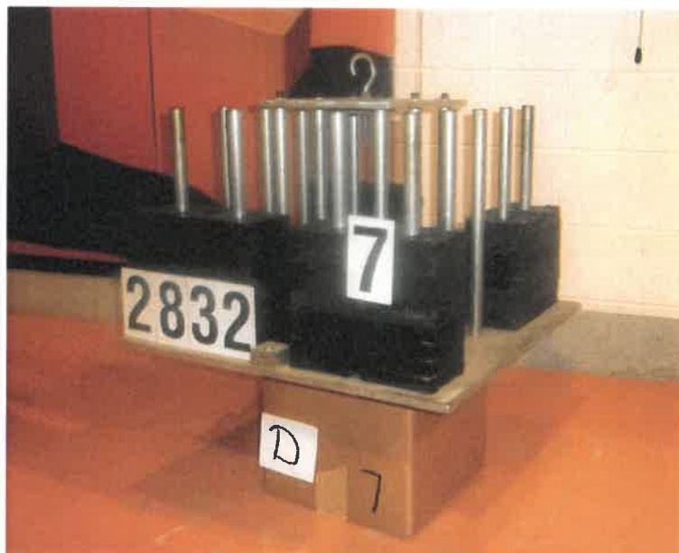
Actual Stack Load of 215.4 kg (475.0 lbs)
