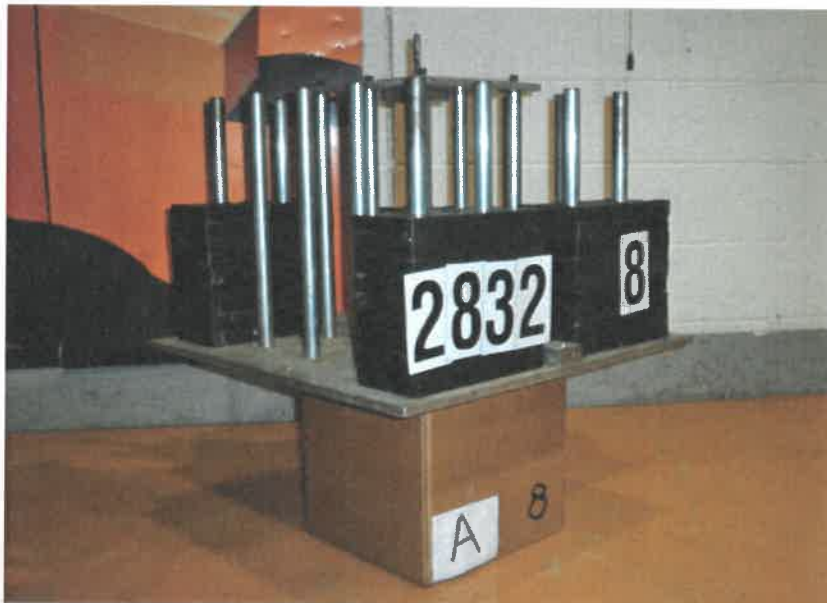
Actual Stack Load of 215.4 kg (475.0 lbs)
