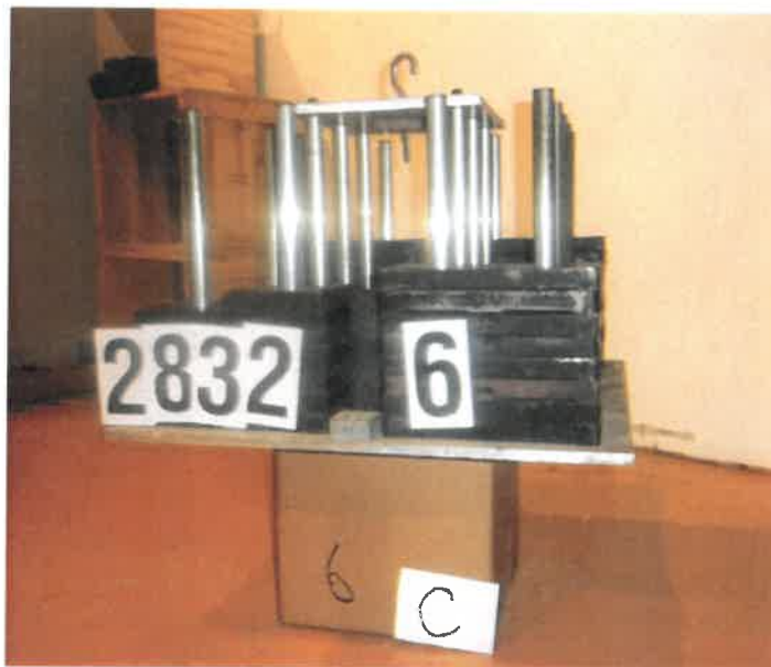
Actual Stack Load of 215.4 kg (475.0 lbs)
