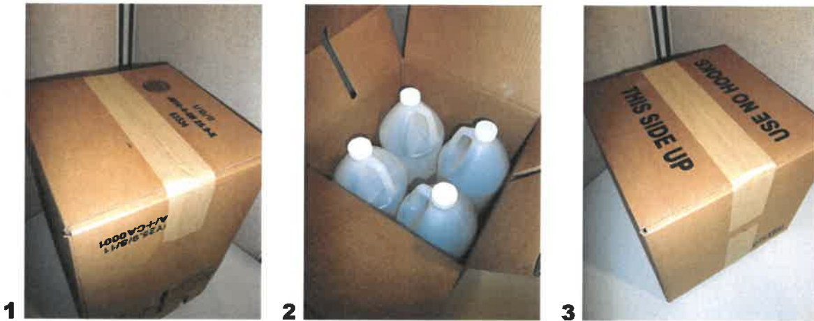
Photo 1: Apply 76mm wide reinforced gummed paper tape, single strip bottom , centered both longitudinally along and spanning the flap seam, extending a minimum of 2-inches onto sides of carton with tape adhered firmly in place. Bottom minor flaps have a 12mm gap when closed, bottom major flaps have a 7mm gap when closed.
