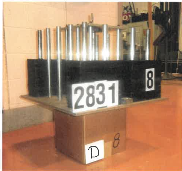
Actual Stack Load of 215.4 kg (475.0 lbs)
