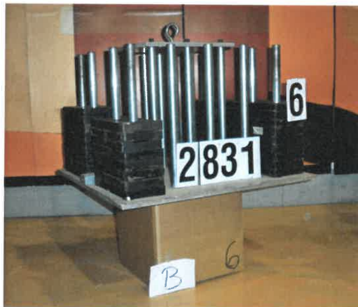
Actual Stack Load of 215.4 kg (475.0 lbs)
