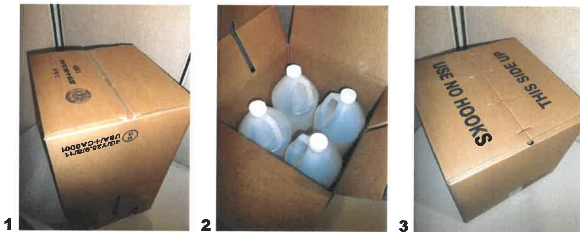
Photo 1: Apply 48mm wide pressure sensitive plastic tape, single strip bottom , centered both longitudinally along and spanning the flap seam, extending a minimum of 2-inches onto sides of carton with tape adhered firmly in place. Bottom minor flaps have a 12mm gap when closed, bottom major flaps have a 7mm gap when closed.
