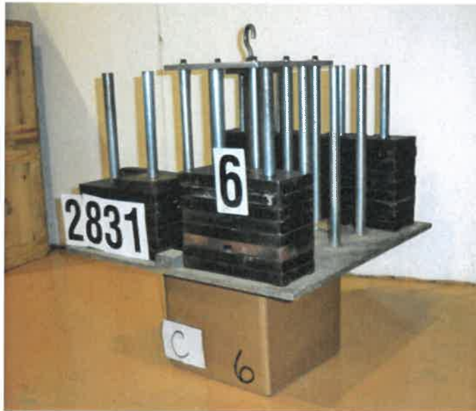
Actual Stack Load of 215.4 kg (475.0 lbs)
